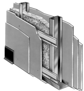
Designing High-STC Wall Partitions: This gypsum board wall assembly uses mass (2 gypsum board layers are on one side, and 3 layers are on the other side), decoupling (resilient channels are screw-attached to the steel studs) and absorption (a layer of mineral fiber insulation is friction-fitted in the partition cavity) to enhance STC performance.
