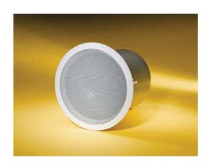
The Lencore Spectra® Sound Masking LG035-M6 is the main unit to the LG035-S6 and duplicates the output of the main. Each main unit consists of an individual self-contained noise generator, audio amplifier, loudspeaker in a damped metal enclosure, powered by 16/18 volts AC transformer and is capable of driving two secondary models.
