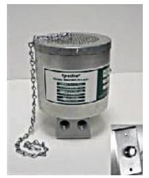
The Lencore Spectra® sound masking LM6-CRCVC unit operates as a central volume control from which global volume adjustments can be made remotely for up to 150 masking units and covering up to 33,000 square feet system-wide. The unit consists of an individual self-contained noise generator, audio amplifier, and loudspeaker in a damped aluminum enclosure, powered by 16/18 volts AC and is capable of driving one secondary model in addition to the aforementioned.
